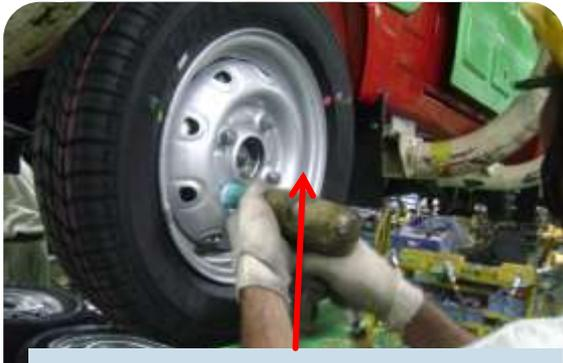
*Auto-Torque regulator to prevent over tightening*
