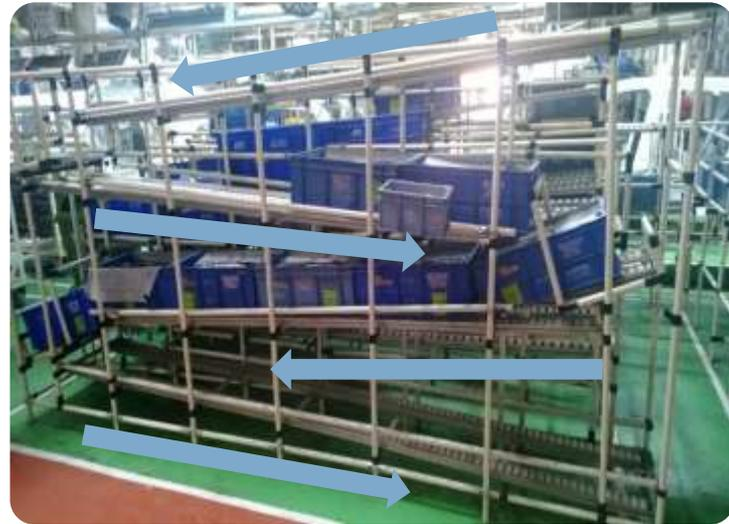
*Tak-a-Tak systems for continuous transfer of material, utilising vertical space, with 'o' manual intervention*
