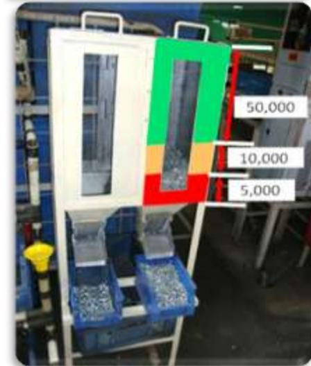
*Hopper systems to ensure **Zero Mix-up** of fasteners*
