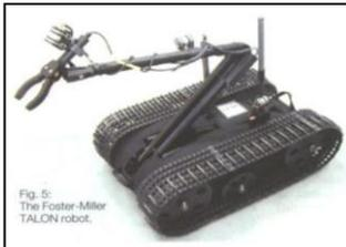
Fig. 5: The Foster-Miller TALON robot.
