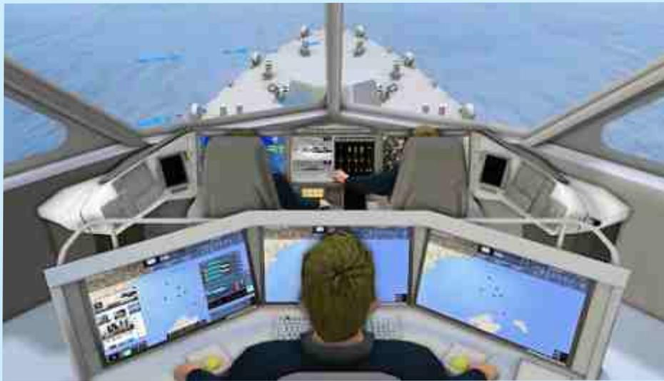
4.19 The architectural base of this system is the SEASTactics, a fully integrated and cost effective solution specifically designed for Patrol Vessels and vessel operating in low intensity warfare scenarios. The SEASTactics provides a common layer for centralized, integrated command and control interface for Navigation, Automation, Communications and Tactical Mission systems (with hardware based on VME technology).
