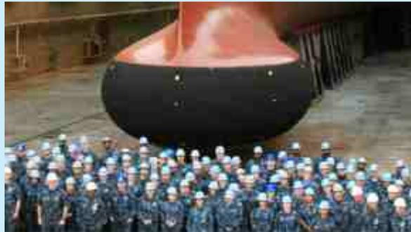
(b) A large bow mounted ship sonar dome [5]
