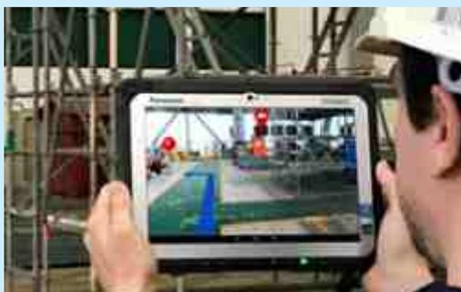
**Fig. 2: Localisation of products inside a workshop using an Industrial Augmented Reality ( IAR) system**
