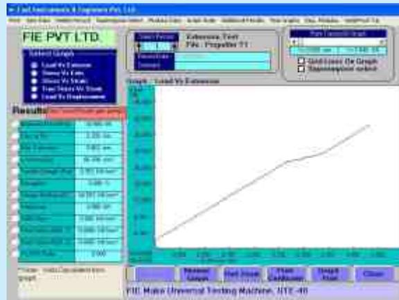
**Table 5 : Tensile test result for UD Pressure Moulding**
