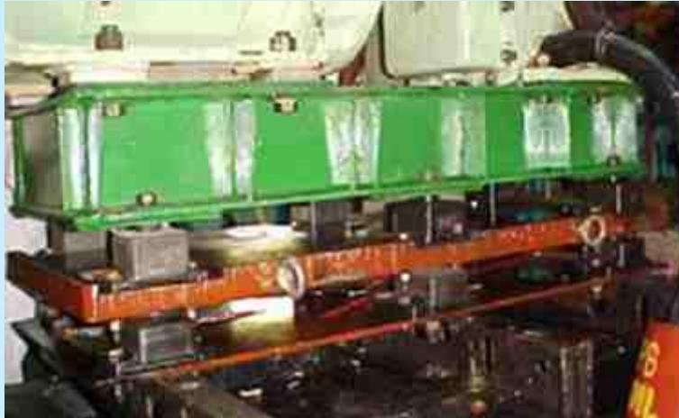
3.2 The hull girder may be treated as the fixed support. Thus the engine mount foundation system can be modelled as a two-degree freedom system with certain assumptions. A two-stage mounting system (raft mounting) is employed where there is a demand for high structure-borne noise attenuation. The main objective of a two-stage mounting system is to reduce vibration levels from machinery to foundation, and thereby to radiate noise levels from ship hull.
