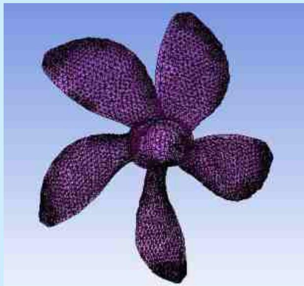
the entire grid was 0.39 million. The quality of the computational meshing grid gets directly influenced by the computation time of analysis and rate of convergence of the cells. Fig 6 shows the grid over the rotating domain. The interfaces have been defined with respect to the stationary domain to get the appropriate results. Fig 7 shows the complete grid over the entire domain for the propeller simulations.
