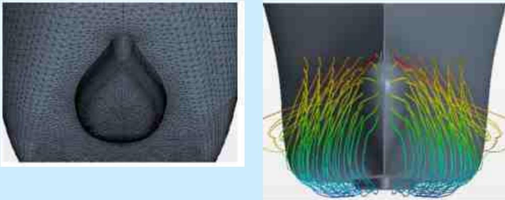
6.2 The results of flow simulation from CFD indicate that the streamlines emanating from the free surface to 1.5m below, are partially effectively diverted towards the sides as desired in the design, and partially pass over the bottom surface.
