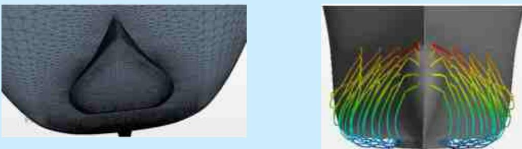
7.2 The results of flow simulation from CFD indicate that the streamlines emanating from the region from free surface to 1.5m below are diverted towards the sides. The streamline pattern around the hull and appendage is shown in Fig.
