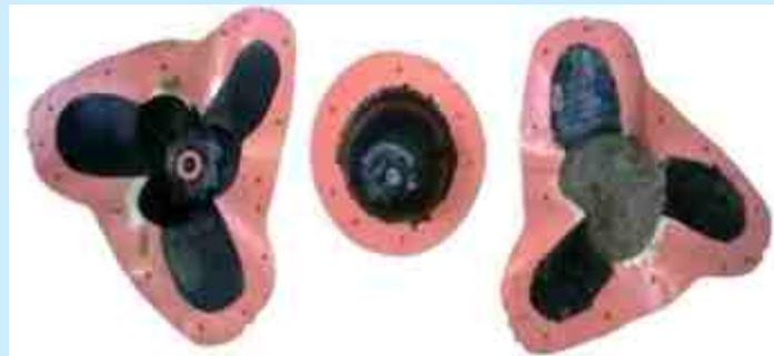
**Fig. 3: Carbon fibre propeller manufactured using hand layup process**
