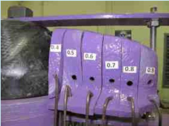
**Fig.7: A view of segment loading for static load test (Ref: 7)**
