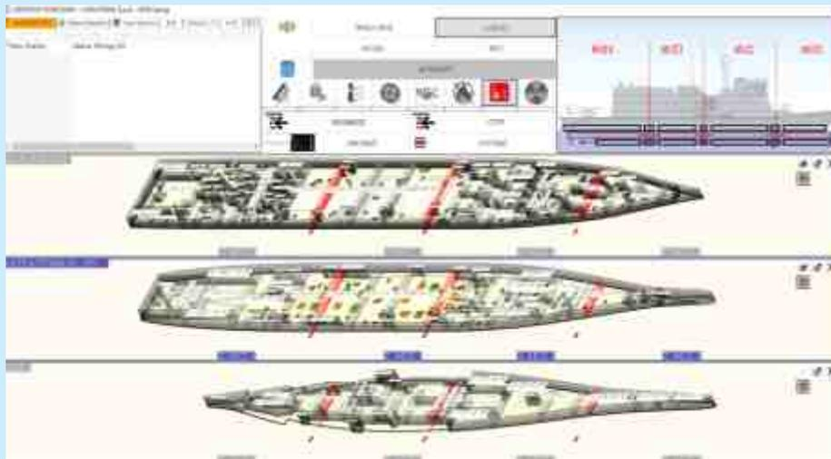
BDCS includes SEASTEMA's own On-Board Stability Software (OBSS) assisting the operator in the management of vessel safety regarding ship stability, both in normal (intact) and emergency (damage) situations:
